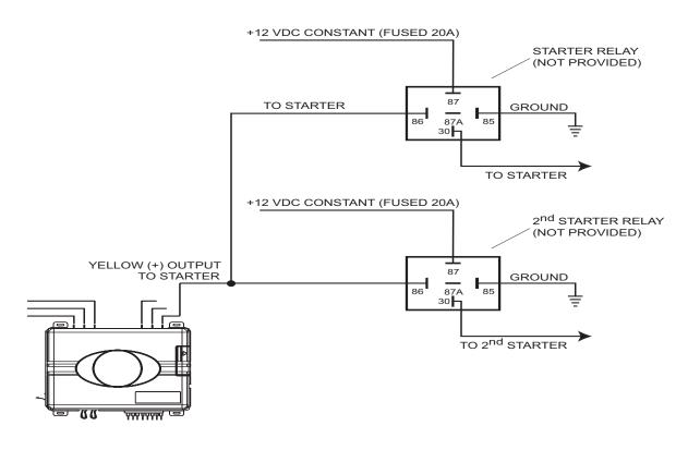
**note!** Always check the Web site information on your vehicle for warnings regarding the starter wire and check engine lights. Some vehicles will trip a check engine light if the starter wire is cut.
